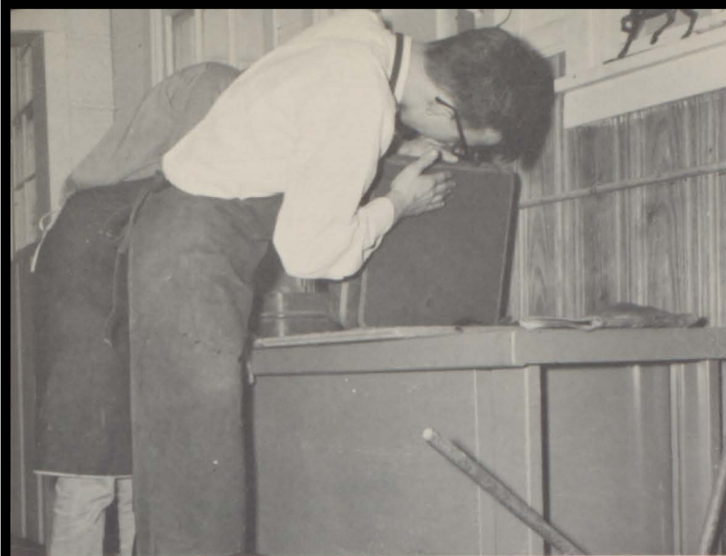
Metalworkers Huel Halliburton preparing a sand mold for casting.
