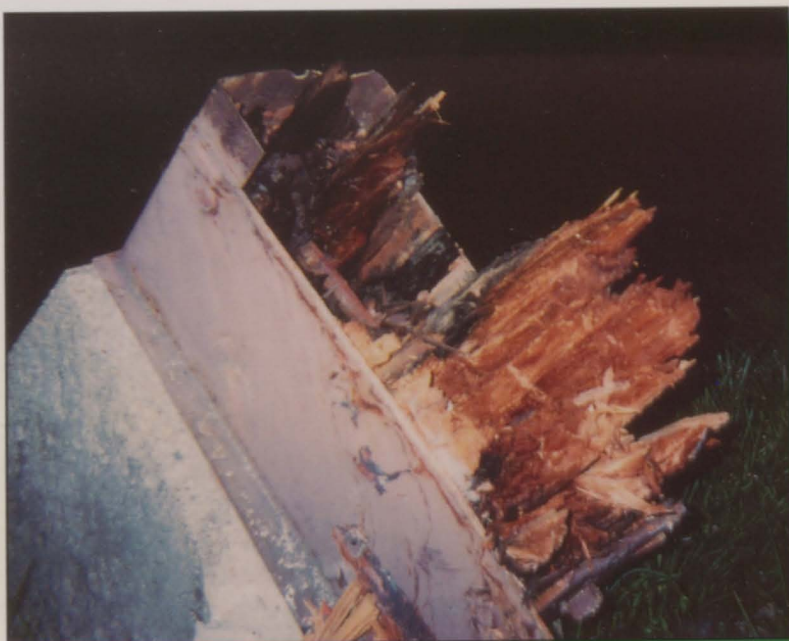
The gym's demise Forty-year-old, rotten wooden beams ultimately reduced roof support, causing structural problems. "I'm glad they caught the problem before it got any worse," said sophomore Ashley Vinson.
